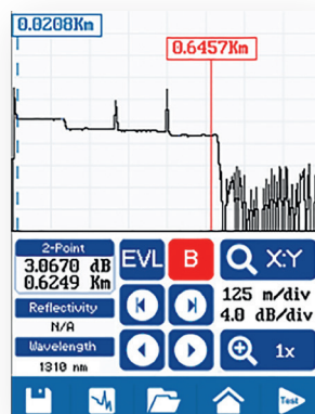
OTDR trace shown for detailed analysis
